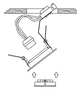
\*Ensure there is adequate free air ventilation around fitting. The nearest illuminated surface must be at least 0.5m distance from the front of the fitting.
